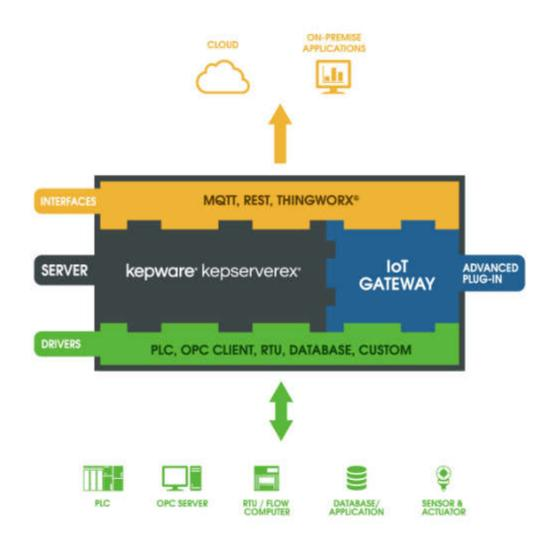
Enterprise and cloud-based solutions enable organizations to search, monitor, analyze, and visualize KEPServerEX-generated data coming from PACs, PLCs, RTUs, flow computers, OPC servers, and other industrial hardware and software. Kepware has partnered with Big Data and analytics providers to enable insight into the operations and conditions of industrial devices and systems.
