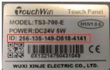
3. When downloading, select the LAN download and scan the IP interface to find the required device ID based on the model and IP address.
