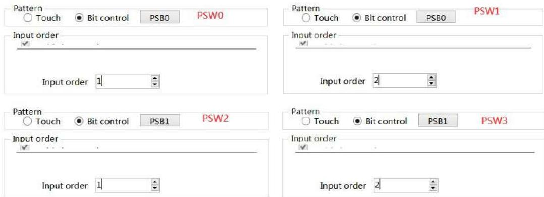
PSW0 and PSW1 are in same group, which are controlled by coil PSB0, and the sequence is 1 and 2 respectively; PSW2 and PSW3 are in same group, which are controlled by coil PSB1 in order of 1 and 2 respectively;
