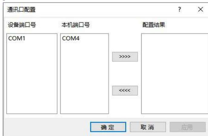
10. At this point, it is necessary to configure the port and connect the device port with the local port. First, click to select the device port number, then click to select the local port number, and then click the middle button. The configuration result will be displayed on the right side.
