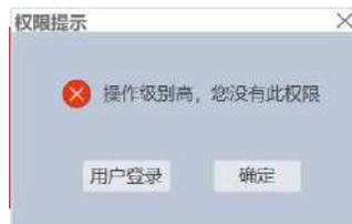
Click the user log in. After logging in successfully, operate the component once. After the first operation, the system automatically cancels the permission limit of the component. Even after logging out, the component can be clicked normally. If the user has logged in, the component will display normally, and clicking the component will not pop up a prompt window.
