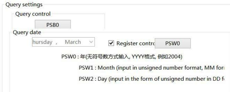
(2) Enter the start time and end time to query in the specified address, set the query control address, and
