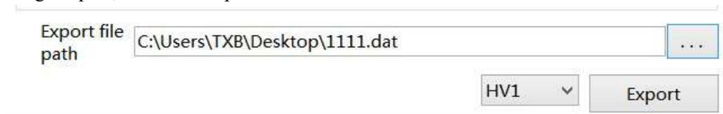
Note: HV1 is an old version and HV2 is a new version. Only HV1 can be selected for the old version of the touch screen, and only HV2 can be selected for the new version of the touch screen. Otherwise, the firmware will be prompted as incorrect. Please refer to 7-3 for the hardware version of the touch screen currently used Device information.
