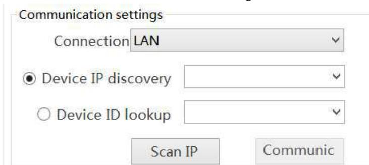
**Device IP discovery:** Input the IP address of the connected HMI, or select the last input address through the drop-down box
