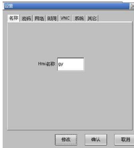
When the modified name is downloaded through the local area network on the download page, scan the IP to display the corresponding name.
