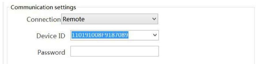
**Device ID:** Input the ID address of the connected HMI, or select the last input address through the drop-down box. The HMI ID can be viewed on the label on the back of the product.
