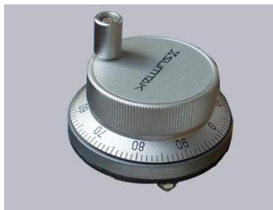
The output signal of the hand pulse generator must be OC (collector open circuit signal) DC24V type. Generally, there will be five wires, three signal wires (A, B, Z), two power wires (24V, 0V), signal wires connected with the corresponding high-speed counting input port of the PLC. The power supply can be supplied by the output 24V of the PLC or by the switching power supply.
