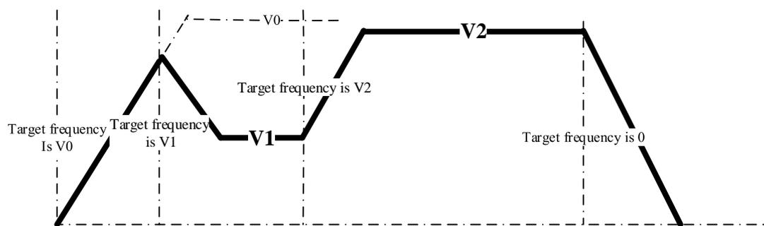
User set target frequency  $V1$  ( $V1 < V0$ ,  $V1 < \text{present frequency}$ ) before reaching setting frequency  $V0$ , at this time, it will go to new setting frequency  $V1$  as the down slope.
