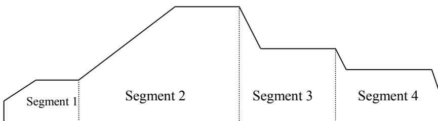
The pulse curve please refer to above diagram. Each segment will send the pulse numbers at setting speed. Except the last segment, each segment includes rising or falling part, stable part. The last segment includes rising part, falling part and stable part.
