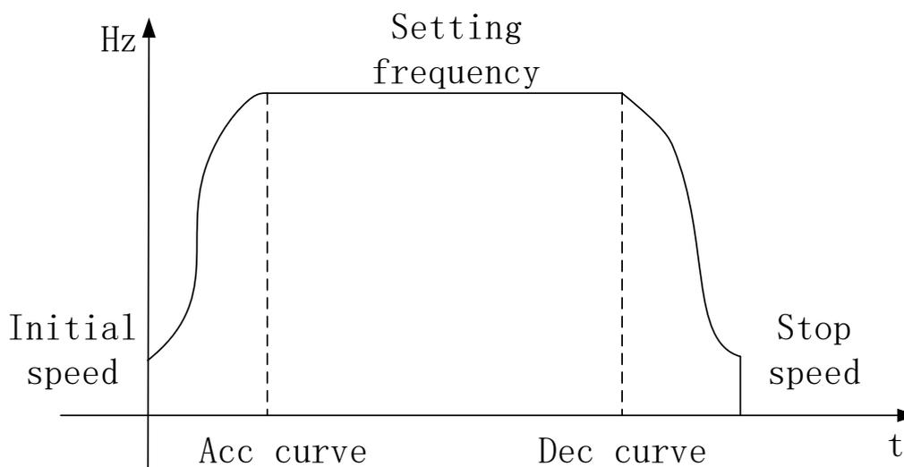
Sine-curve mode is fit for the receiving of stepper motor and servo motor and improve the run performance of stepper motor and servo motor. The details please refer to S-curve acceleration and deceleration.
