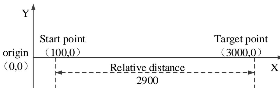
**Pulse coordinate diagram**
