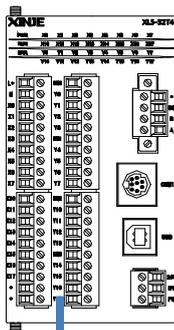
**Transistor output (Y0, Y1, Y2, Y3)**
