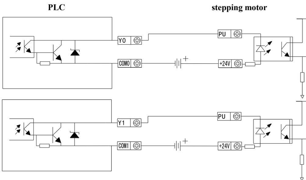
Note: If the pulse and direction terminals of the stepper motor are driven by DC5V, please connect 2.2K Ω resistance behind the pulse and direction terminals.
