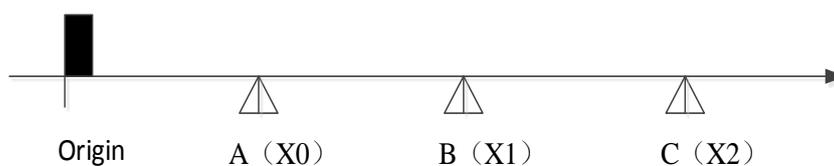
As the above diagram, it needs to move three segments of distance, the position of A, B, C is unknown and the moving speed is different for each segment. We can configure the PLSR to do it. First we install proximity switch at point A, B, C and connect to PLC input X0, X1, X2. The pulse output terminal is Y0, the direction terminal is Y2.
