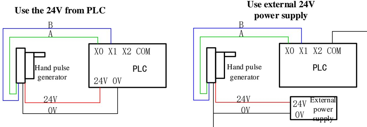
Note: When using external switching power supply, the COM of PLC input should be short connected with 0V.
