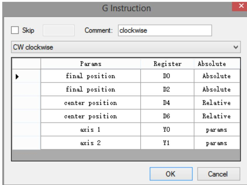
In the register list, double click the value can change the register address and axis output terminal.
