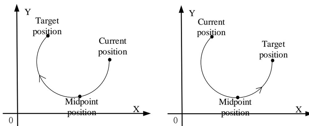
When the target position is set to the same position as the current position (that is, two points become a point), the next circle can not be determined by two points (in three points, as long as two points coincide or three points are in a straight line, it can not form an arc), so this mode can not draw a whole circle. Three-point arc interpolation ARC has three modes, the following will be used one by one.
