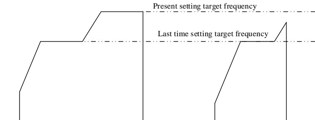
When the present frequency is changed, it will accelerate/decelerate to target frequency as rising/falling slope.
