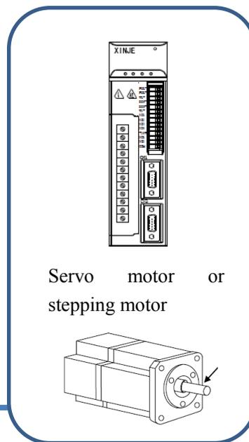
※: 4-axis servo motor or stepping motor can be controlled.
