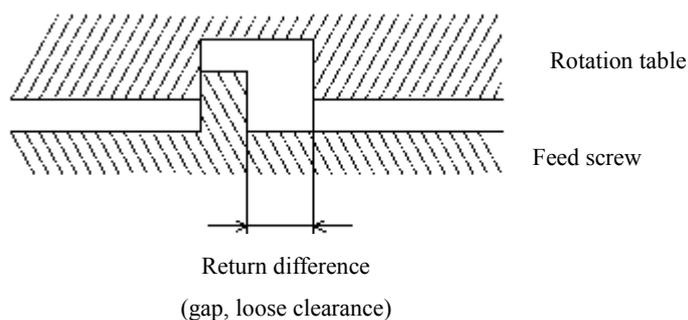
The table moves from left to right, when the table right side moves to position A, it will stop and moves from right to left. As the ball screw clearance, it cannot move left for some pulses, and the actual moving distance is less than setting value. If there is no clearance, it will move from A to B. in order to delete the error, we must send some pulses before moving left, and then send the actual moving left pulses.
