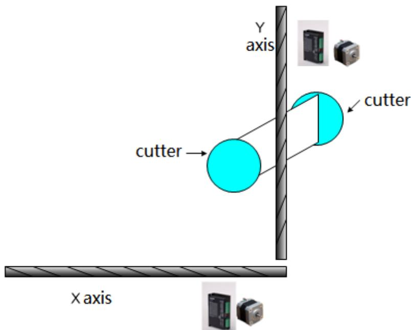
As shown in the figure, two stepper motors control X and Y axis respectively, and use the arc interpolation instruction of XINJE XDM PLC to make X and Y axis coordinate and get out of the circular arc track. The relative distance of the cutter installed on the workbench determines the width of the plate cut by the cutter.
