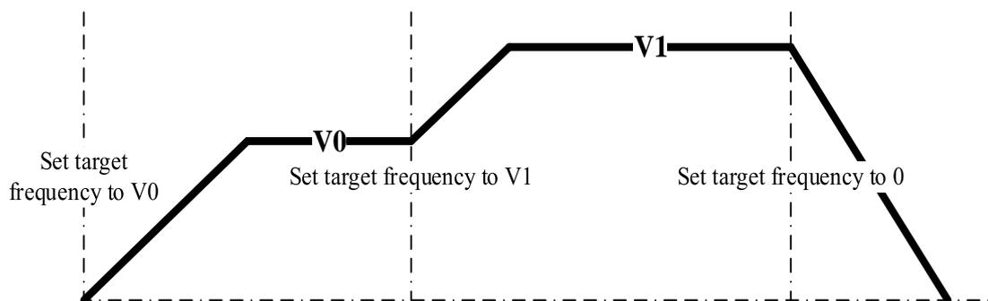
(2) the pulse is not in stable segment when user setting new frequency, it will switch to setting frequency through the slope. (present setting frequency > last time setting frequency, takes present setting frequency as target).
