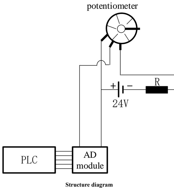
For example: the output signal of potentiometer is shown as below:
