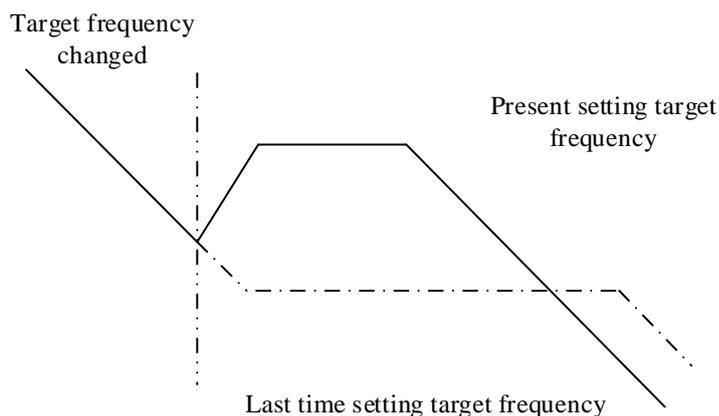
When the present pulse frequency is changed by user, PLC will calculate the pulse curve again, then output pulse as the new pulse curve.
