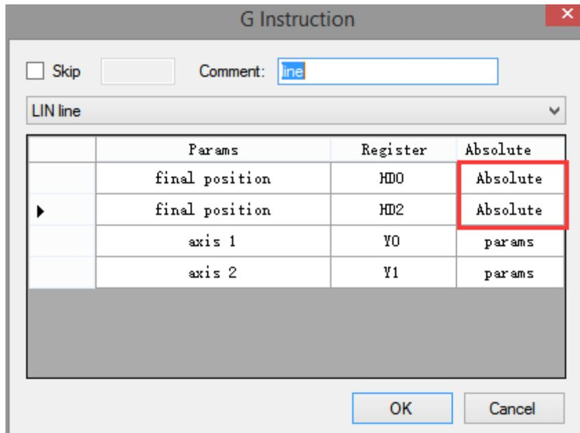
Double-click the "parameters" to configure the parameters of Y0 and Y1 axis [pulse direction terminal], [group 2 parameters - pulse default speed (Hz)], [group 2 parameters - pulse default speed acceleration time (ms)], [group 2 parameters - pulse default speed deceleration time (ms)], as follows:
