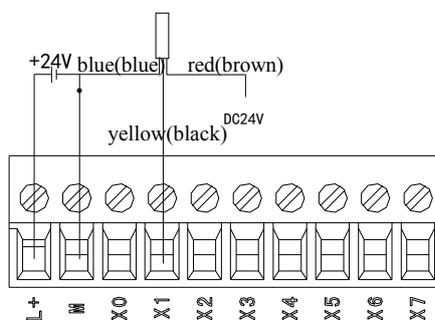
Three-wire (NPN) proximity switch wiring
