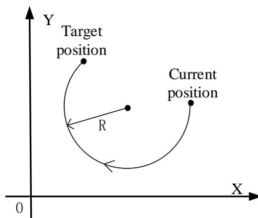
With the above figure, when the target position is set at the same position as the current one, the next circle can not be determined, so this mode can not draw a whole circle. There are three modes of CW\_R. The usage of CW\_R is described below.
