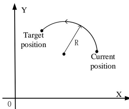
With the above figure, when the target position is set at the same position as the current one, the next circle can not be determined, so this mode can not draw a whole circle. There are three modes of CCW\_R. The usage of CCW\_R is described below.
