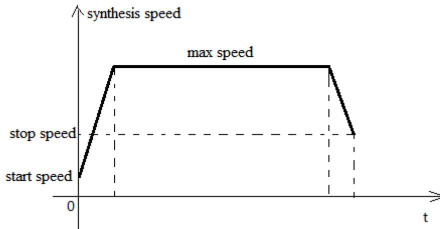
When there are multiple continuous linear/arc interpolation instructions and the speed between them needs to be constant and jump directly, the stop speed and maximum speed of the previous linear/arc interpolation can be set the same as the start speed and maximum speed of the next segment.
