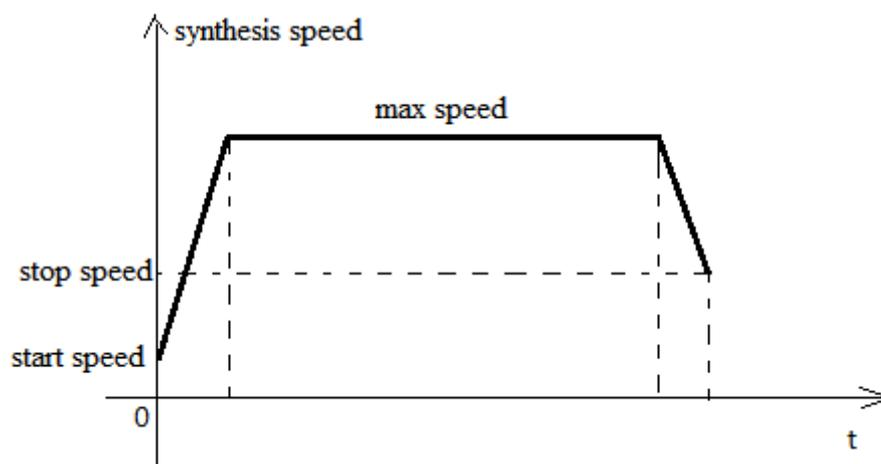
When there are multiple continuous linear/arc interpolation instructions and the speed between them needs to be constant and jump directly, the termination speed and maximum speed of the previous linear/arc interpolation can be set the same as the starting speed and maximum speed of the next segment.
