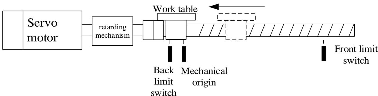
Positive: the work table will move in forward direction when executing ZRN.
