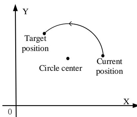
With the above image, when you need to draw an entire circle, just set the target position to the current position. There are three modes of anticlockwise arc interpolation CCW, the usage of which is described below.
