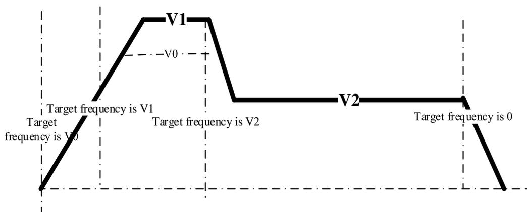
User set target frequency  $V1$  ( $V1 > V0$ ) before reaching setting frequency  $V0$ , at this time, it will go to new setting frequency  $V1$  as the slope.
