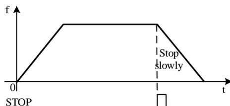
According to the descending slope, the current pulse frequency of the pulse falls to the pulse stop frequency or the number of pulses in the pulse section is all sent out and stop the pulse output.
