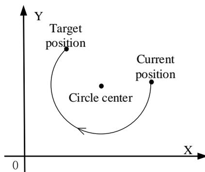
From the above figure, we can see that when we need to draw a whole circle, we only need to set the target position to the current position. CW has three modes. The usage of CW is described below.
