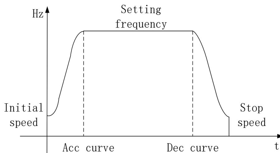
Sine curve mode: the speed changing for accelerating or decelerating is sine curve.
