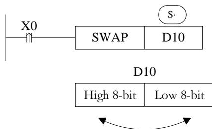
Exchange the high 8-bit and low 8-bit of 16-bit register.
