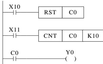
The counter C0 increases one when the X11 drives once. When C0 value reaches 10, the output acts. Then X11 drives again, C0 will continue increase one.
