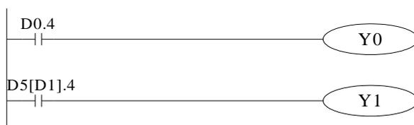
D0.4 means when the fourth bit of D0 is 1, set Y0 ON.
