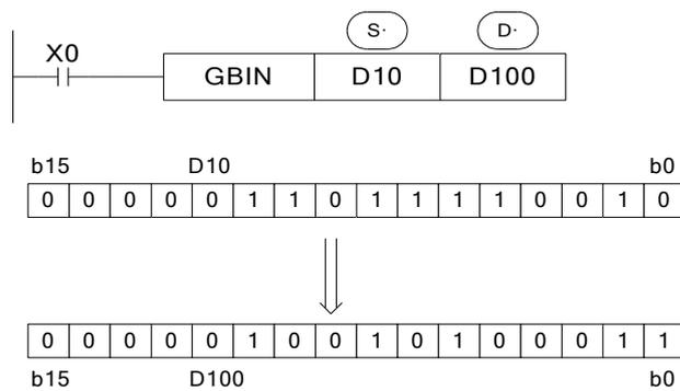
From the left second bit of D10, XOR each bit with the value after decoding, as the bit value after decoding (the left bit will not change). The transformation value will be stored in D100.
