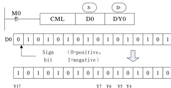
Each data bit in the source device is reversed (1→0, 0→1) and sent to the destination device. If use constant K in the source device, it can be auto convert to be binary. This instruction is fit for PLC logical converse output.
