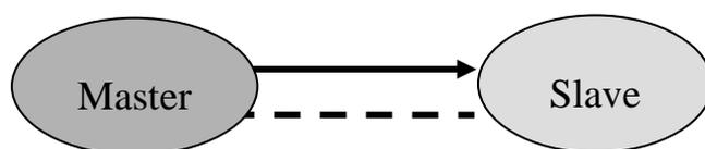
There is dotted line in the diagram. It means any PLC can be master station when all PLC in the network don't send data. As the PLC do not have unified clock standard, communication will fail when more than one PLC send data at one time. It is not recommended to use.
