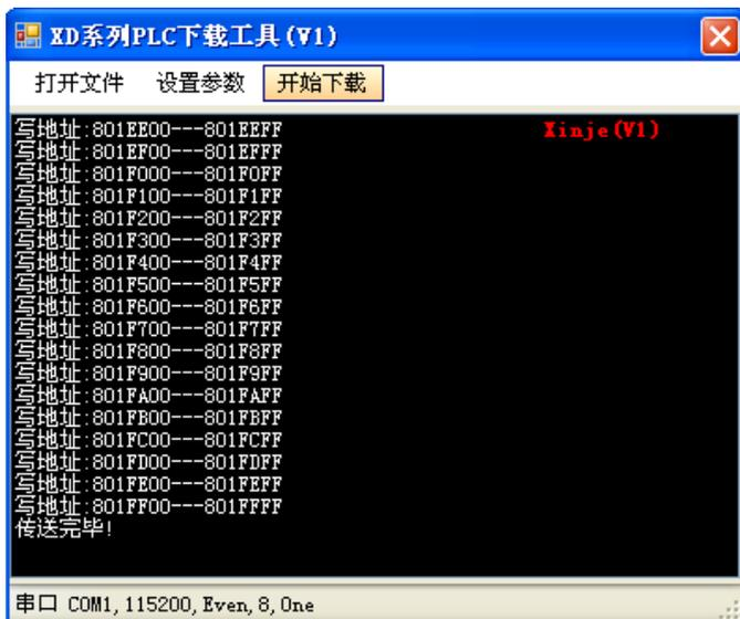
After finishing the update, cut off the PLC power, take off the short jumper, then power on the PLC again.
