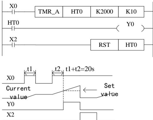
If `X0` is ON, `HT0` accumulates the 10ms pulse based on the current value. When the accumulation value reaches the set value `K2000`, the timer output activates.
