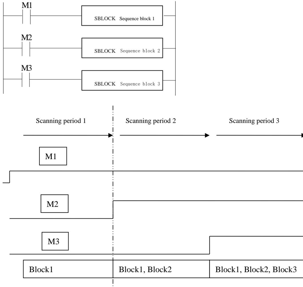
Note: When the program in the BLOCK is not executed and the triggering condition M is disconnected, the BLOCK will not stop immediately, but will complete the last scan, and will stop after the rest of the program has been executed.
