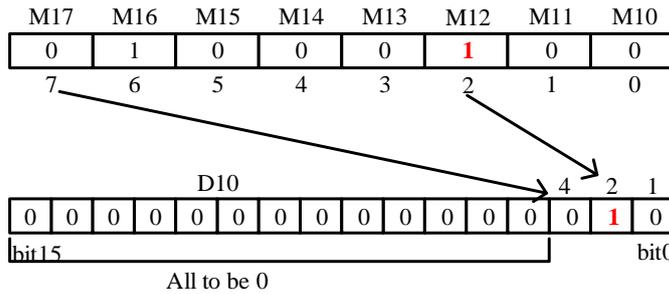
If the number of bits in the source address is 1, the high bit side is ignored, and if the source address is 0, the instruction will not be executed.
