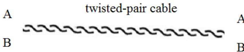
Connect all A terminals, connect all B terminals. A is RS485+, B is RS485-.
