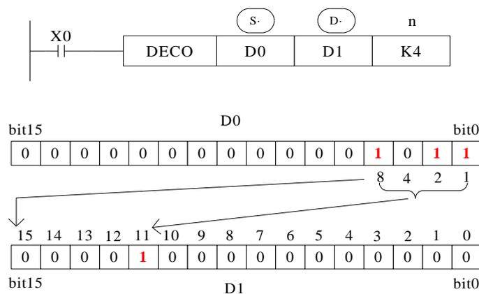
The low  $n$ -bit ( $n \leq 4$ ) of the source address is decoded to the target address. When  $n \leq 3$ , the high 8-bit of the target turns to 0.
