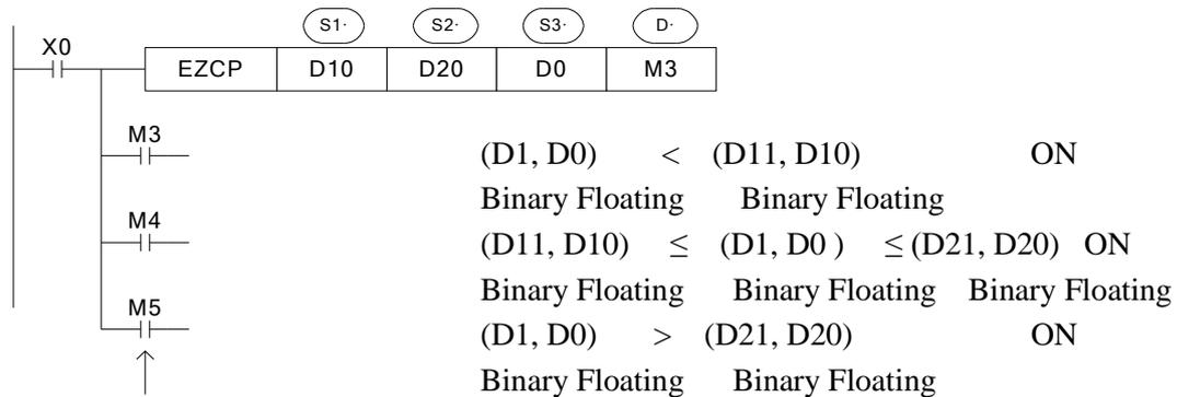
When X0 is OFF, even EZCP doesn't run, M3~M5 will keep the status before X0 is OFF.
