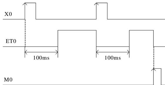
When the pre-condition of STR is normally open/closed coil, the precise timer will set ON immediately when the timing time arrives and reset the timing, and cycle back and forth.
