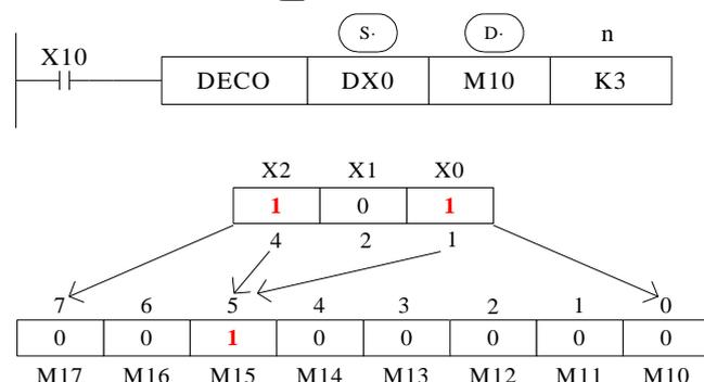
$N = 3$ , so the decoding object is the lower three bits in DX0, which are X2 ~ X0.
