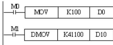
When M0 is ON, write 100 into D0.(16 bits value)
