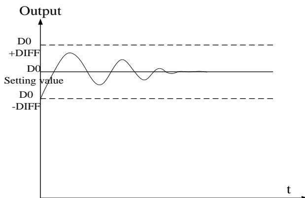
To enter the auto tune mode, please set bit7 of (S3+ 2) to be 1 and turn on PID working condition. If bit8 of (S3+ 2) turn to 1, it means the auto tune is successful.
