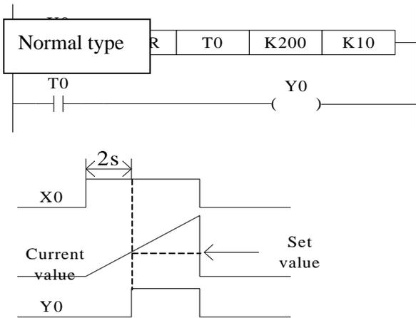
If `X0` is ON, then `T0` accumulates 10ms pulse based on the current value; when the accumulation value reaches the set value `K200`, the timer output activates. I.e. the output activates 2s later. If `X0` is OFF, the timer resets, the output resets;
