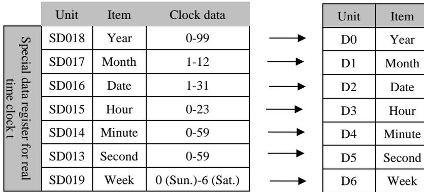
The RTC (real time clock) value is in BCD code format (SD013 to SD019). Please choose hex format to monitor the RTC value in XDPpro software. The value can be transformed to decimal format by BIN instruction. After reading the RTC by TRD instruction, the value will show in decimal format.
