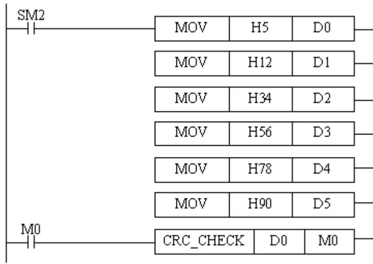
Download to PLC, then RUN PLC, set M0, via Free Monitor, we can find that values in D6 and D7 are the highest and lowest bit of CRC parity value;
