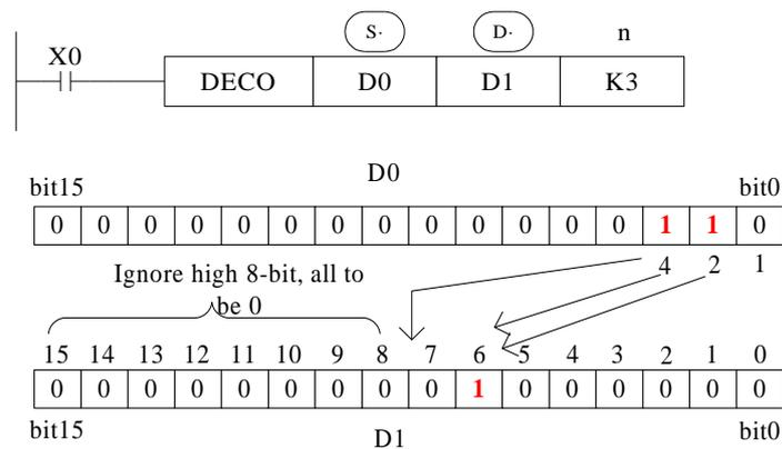
The low  $n$ -bit ( $n \leq 4$ ) of the source address is decoded to the target address. When  $n \leq 3$ , the high 8-bit of the target turns to 0.
