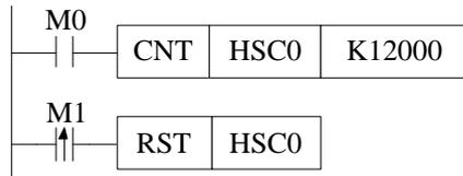
As shown above, when M0 is ON, HSC0 begins to count the pulse input of X0 port; when M1 changes from OFF to ON, HSC0 is reset, and the count value in HSCD0 (double words) is cleared.
