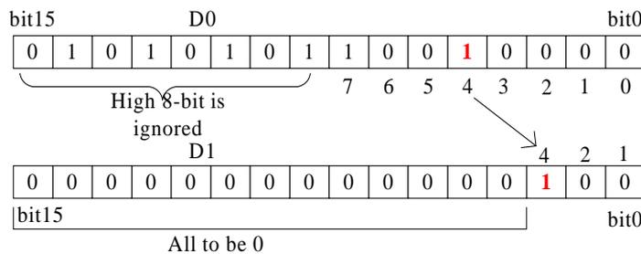
If multiple bits in the source address is 1, the high bit side is ignored, and if the source address is 0, the instruction will not be executed.
