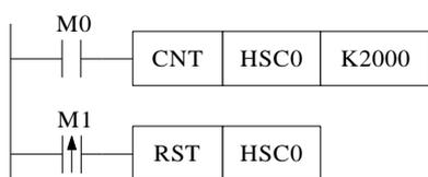
When the M0 is ON, HSC0 counts the rising edge of the OFF to ON of the input X0 port at high speed.
