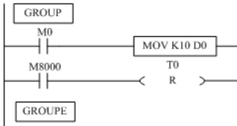
Generally, GROUP and GROUPE instruction can be programmed according to the group's function. Meantime, the programmed instructions can be FOLDED or UNFOLDED. To a redundant project, these two instructions are quite useful.
