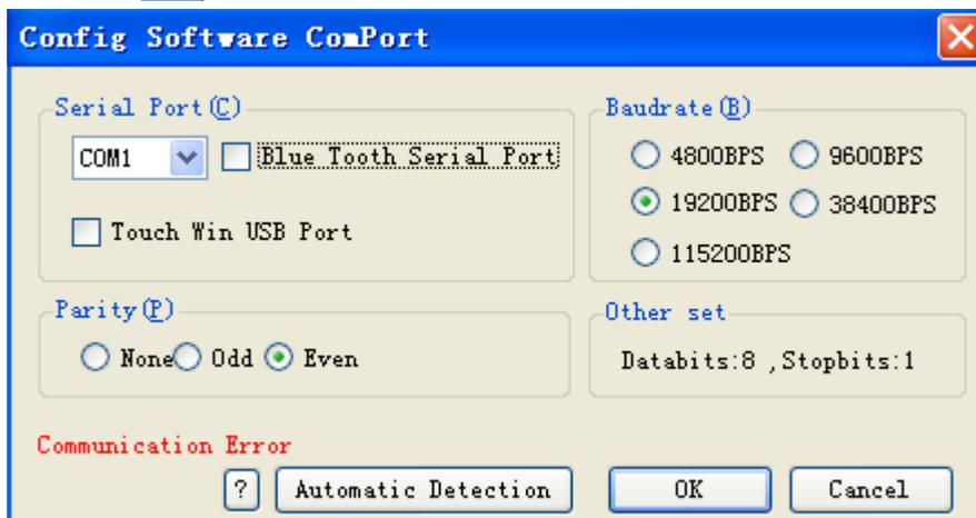
Choose correct communication serial port according to your PC actual serial port.; baud rate selects 19200BPS, parity check selects even parity, 8 data bits, 1 stop bit; you can also click 'check' button directly in the window, and communication parameters will be selected by PLC itself. 'Connect PLC successfully' will be displayed on the left bottom of window as below:
