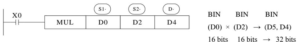
The contents of the two source devices are multiplied together and the result is stored at the destination device in the format of 32 bits. As the above chart: when (D0)=8, (D2)=9, (D5, D4)=72.
