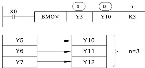
As the following picture, when the data address overlapped, the instruction will do from 1 to 3.
