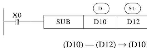
(S1) appoint the soft unit's content, subtract the soft unit's content appointed by (S2) in the format of algebra. The result will be stored in the soft unit appointed by (D) (5-(-8)=13) The action of each flag, the setting method of 32 bits operation's soft units are both the same with the preceding ADD instruction.
