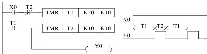
X0 is ON, Y0 begin to twinkle. T1 is Y0-OFF time; T2 is Y0-ON time.
