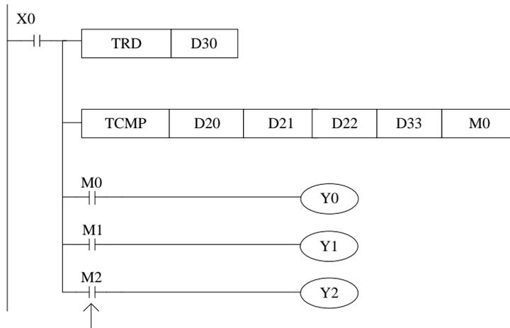
The present clock is 15:32:49 7,30,2014 Wednesday. So D30=14, D31=7, D32=30, D33=15, D34=32, D35=49, D36=3. If the setting time is 15:32:49, D20=15, D21=32, D22=49, so Y1=ON. If the setting time is 17:32:49, D20=17, D21=32, D22=49, so Y0=ON. If the setting time is 2:32:5, D20=2, D21=32, D22=5, so Y2=ON.
