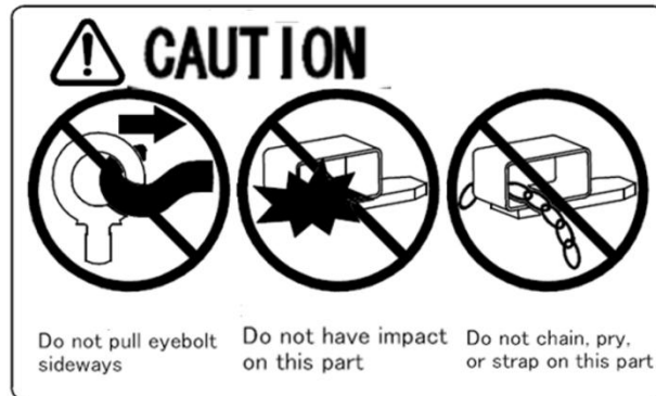
Figure 91 Precautions for the manipulator during handling
