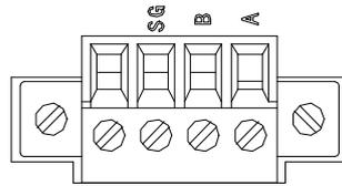
When using RS485 communication, please use twisted pair (as shown below), if conditions permit, shielded twisted pair cables can be used and grounded at a single end. If there is no reliable ground, they can also be suspended.
