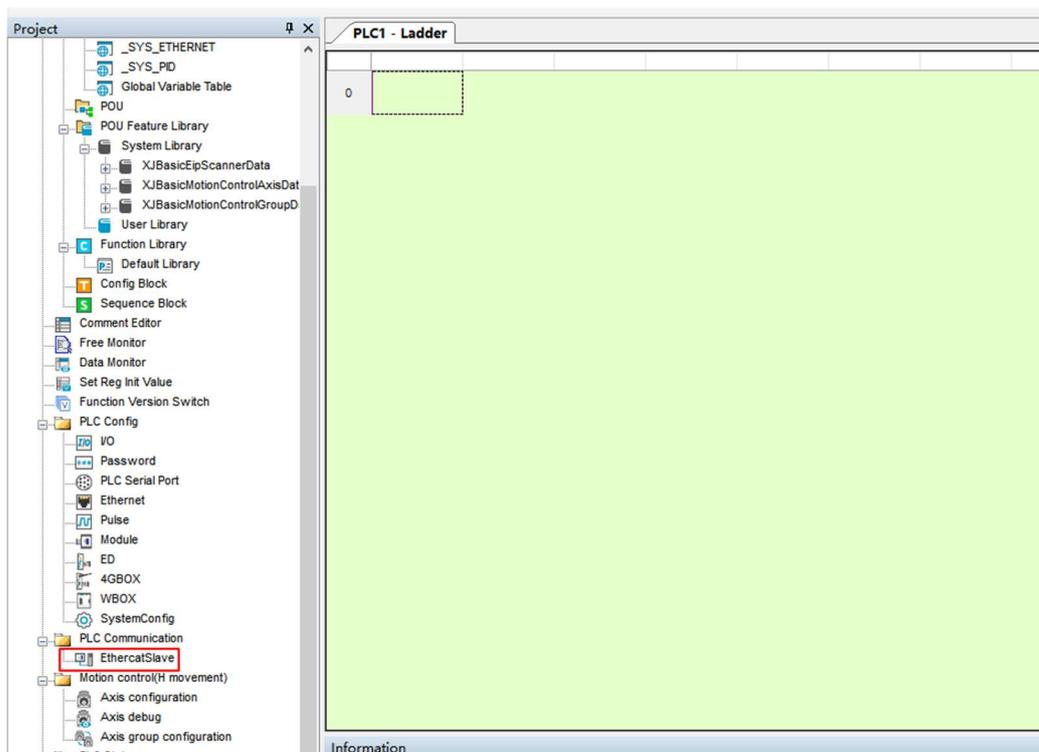
2. Configure data transmission in the slave PLC configuration interface, add the first data connection, select the "master<-- slave" direction for transmission, assign PDO to # x1A00, select sub index # x01, select D0 as the starting address, and have a length of 10. Add the second connection, select the "master -->slave"
