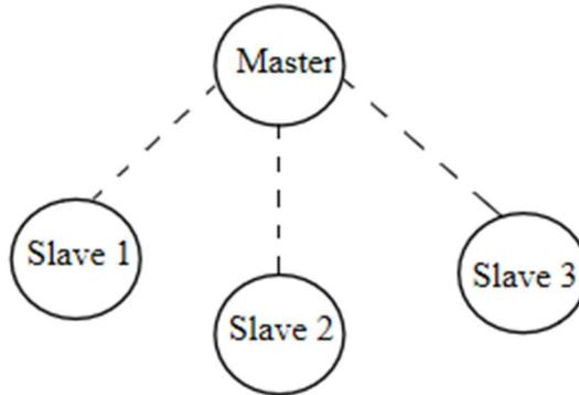
In the RS232 network (as shown below), only one-on-one communication is allowed, and there is only one master and one slave at a certain time.
