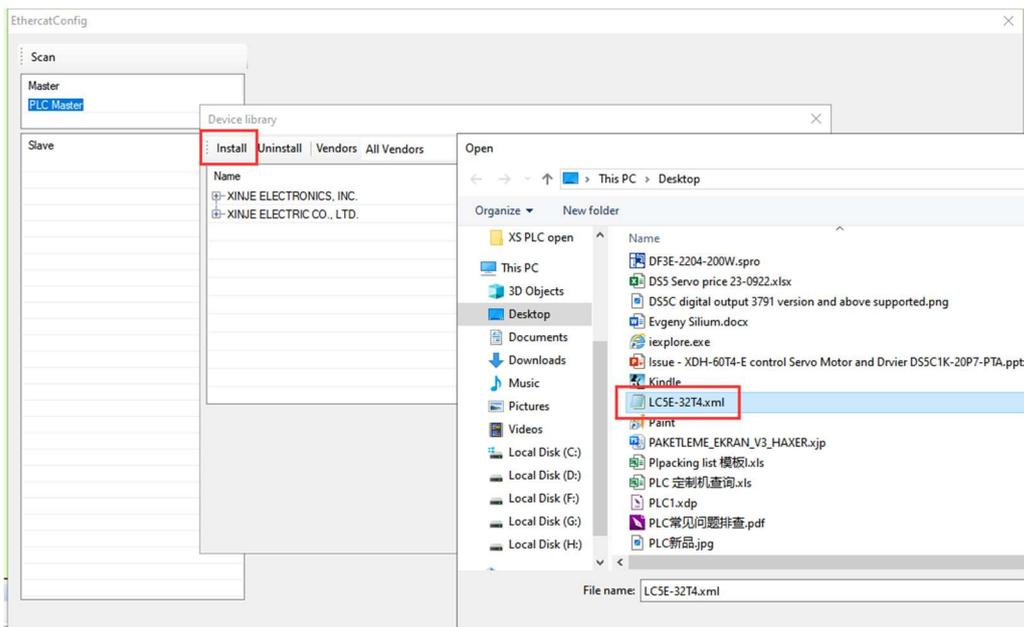
2. Scan the slave station and confirm the PDO parameter configuration on the expert process data interface, since the slave station is configured with # x1600 and # x1A00, selecting these two parameters in the master station configuration will suffice (If adding other PDO parameters from the station, you can check the other PDO parameters). Configure write activation.
