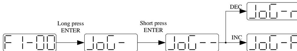
During jog operation, parameters such as gain will participate in the control, and whether the parameter setting is appropriate can be judged according to the operation condition.
