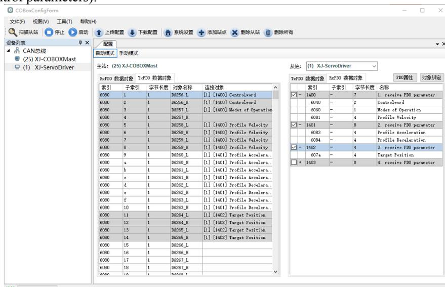
② Download and activate the configurations. The slave station state machine automatically switches from PreOP to OP state. At this time, SDO and PDO can receive and send signals. XDPpro allows you to monitor or modify the mapping of the object dictionary. The specific correspondence is shown in the figure below.
