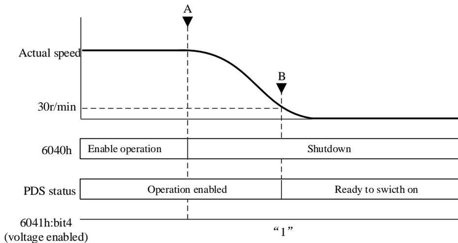
Note: 6041h: bit4 (statusword: voltage enabled) is still 1 and does not change.
