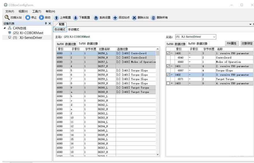
② Download the activation configuration, and the slave state machine will automatically switch from PreOP to OP state. At this time, SDO and PDO can receive and send signals. The mapping of object dictionary can be monitored or modified through XDPpro software. The specific correspondence is shown in the figure below.
