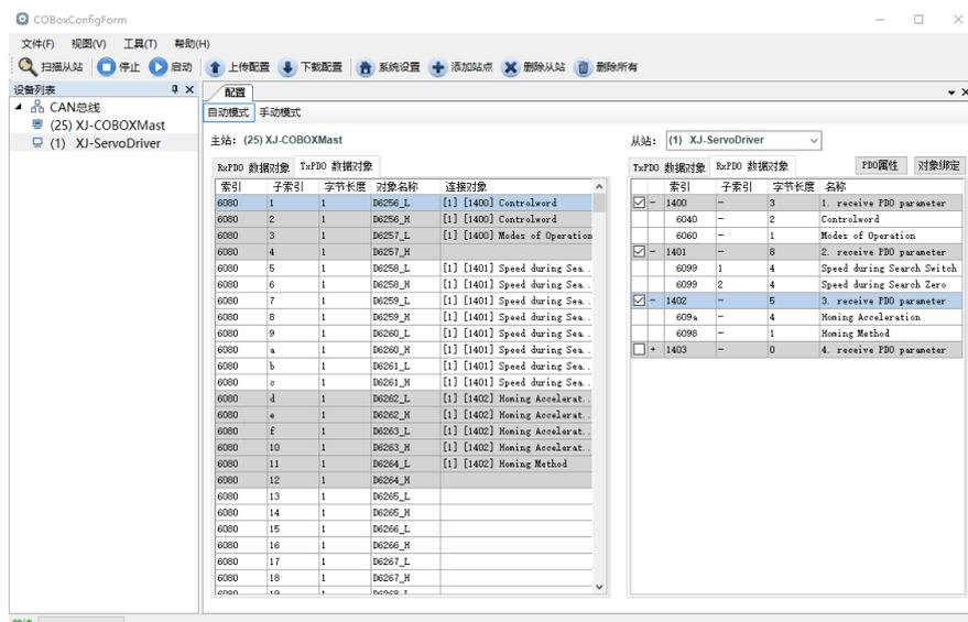
③ Download and activate the configuration, and the slave state machine will automatically switch from PreOP to OP state. At this time, SDO and PDO can receive and send data. The mapping of the object dictionary can be monitored or modified through XDPpro software. The specific correspondence is shown in the figure below.
