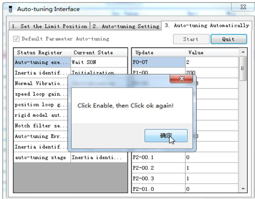
8. The upper device starts to send pulses, wait the completion of auto-tuning.
