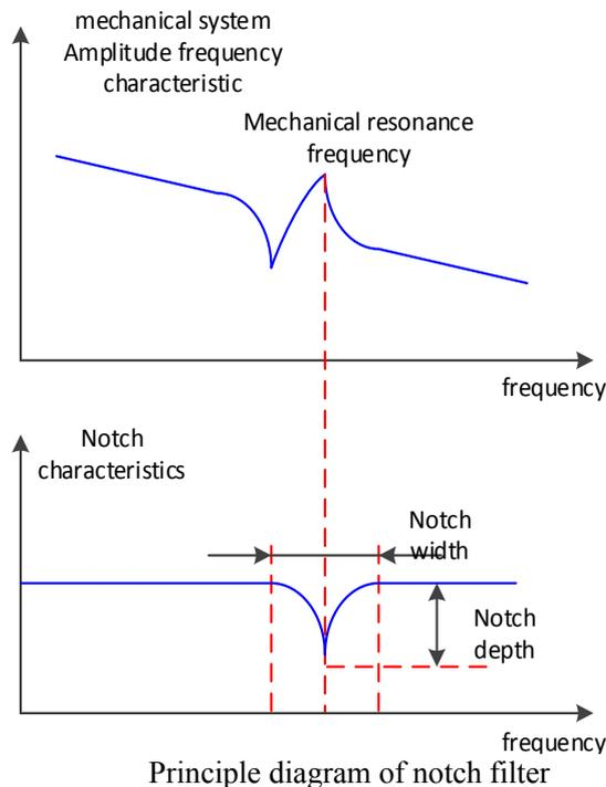
The servo driver has five sets of notch filters, each with three parameters, notch frequency, notch attenuation and notch bandwidth. The first and second notches are set automatically, and the third, fourth and fifth are set manually. The torque instruction filter and notch filter are in series in the system. As shown in the figure below, the switch of the notch filter is controlled by P2-69 and P2-70.
