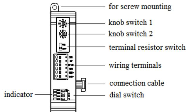
Knob switches 1 and 2 are used to set the node address (i.e. station number) of XD-COBOX-ED module in CANopen network.
