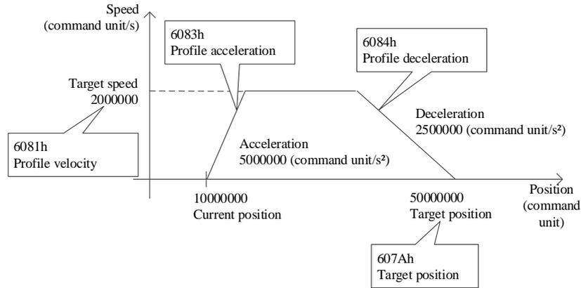
The relative mode or absolute mode can be determined by bit6 (absolute / relative) of 6040h (control word).
