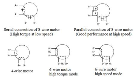
The method to judge whether the series connection or parallel connection of stepper motor is correct or not: rotate the motor shaft directly by hand without connecting the driver. If it can rotate easily and evenly, it means that the wiring is correct. If it encounters large resistance and uneven and accompanied by certain sound, it means that the wiring is wrong.
