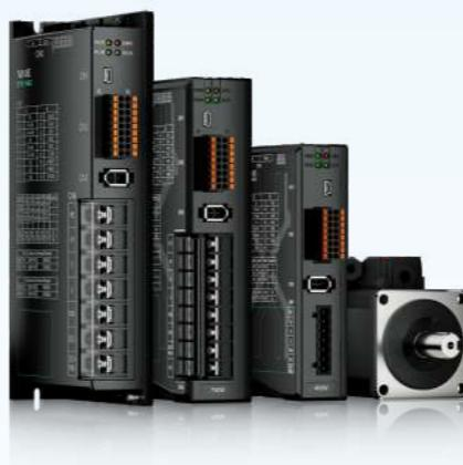
The low-voltage servo system currently has one subseries of bus type, with a compact design, lightweight and compact body, rich interfaces, support for communication protocols such as CANopen and Modbus, low-voltage DC power supply, built-in 24V brake power output, and gain adjustment in just three steps, reducing debugging time.
