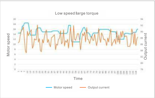
When the VH6 series frequency converter drives the motor at 0.5Hz, the torque output is as high as 180%, reflecting the strong low-frequency torque performance.
