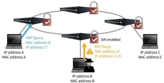
DAI validates the ARP packets in a network. DAI intercepts, logs, and discards ARP packets with invalid IP-to-MAC address bindings. This capability protects the network from some man-in-the-middle attacks.
