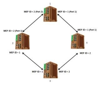
The MEP ID in a link connection should be the same. For the example above the ERPS Ring, the port 1 from device one, the MEP ID is 1 and the port 1 from device 4, the MEP ID is also 1. In one device the MEP ID cannot be the same, it can be used only for a port. Below is the CFM CCP configuration page. In this page user may configure the Maintenance Domain, Maintenance Association and the Maintenance association End Point setting.
