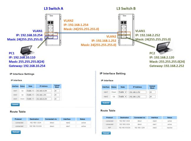
1. Apply IP address, Subnet Mask for the two VLANs and check the Route Table.
