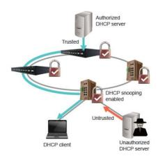
DAI validates the ARP packets in a network. DAI intercepts, logs, and discards ARP packets with invalid IP-to-MAC address bindings. This capability protects the network from some man-in-the-middle attacks.
