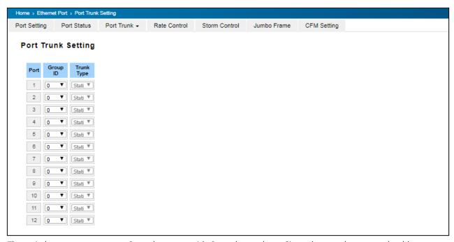
The switch can support up to 8 trunk groups with 2 trunk members. Since the member ports should use same speed/duplex, max trunk members would be 8 for 100Mbps, and 2 members for Gigabit.
