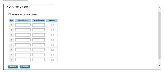
WoMaster' Switches support a useful function that help user to maintain the PD's status and help use to saving the maintenance time and money. Once user defined this function, the PoE Switch will request PD system and turn-off PoE power if PD system does not echo the request. After the duration time (cycle time), the PoE switch will start request PD again.
