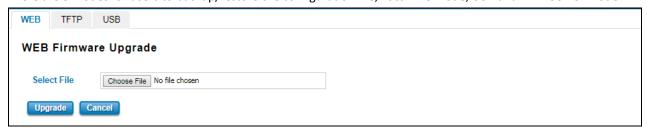
**Web** mode: The switch acts as the file server. Users can browse the target folder and then type the file name to back-up the configuration. Users also can browse the target folder and select the existed upgrade file. This mode is only provided by Web UI while CLI is not supported.
