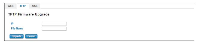
**TFTP Server** mode: In this mode, the switch acts as the TFTP client. Before do so, make sure that TFTP server is ready. Then please type the IP address of TFTP Server and Backup configuration file name. This mode can be used in both CLI and Web UI.
