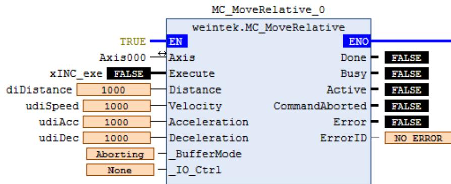
**Position:** Specify the target position, which equals to current position + specified distance.
