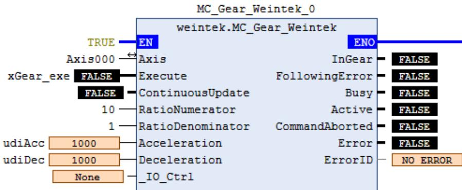
ContinuousUpdate: When it is TRUE, velocity can be updated continuously when the axis is in motion.
