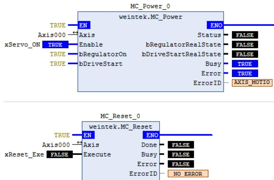
When an error occurs, MC\_Power.Error=TRUE, please execute MC\_Reset to change the axis state from Errorstop to Standstill, to continue operation.
