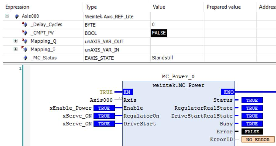
As shown in the figure above, after triggering MC\_Power.Enable, MC\_Status enters Standstill state, which means the axis is ready for motion instructions.
