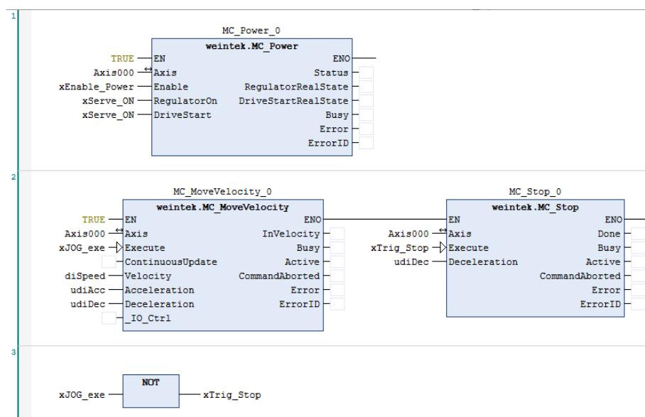
The following three function blocks are used for JOG operation:
