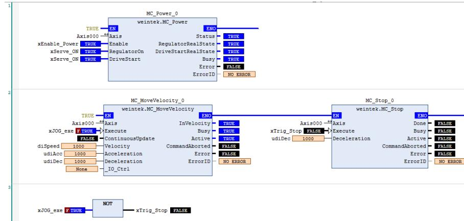
Press xPEnable\_Power & xServe\_ON button to execute MC\_Power function block to start iR-PU01-P.
