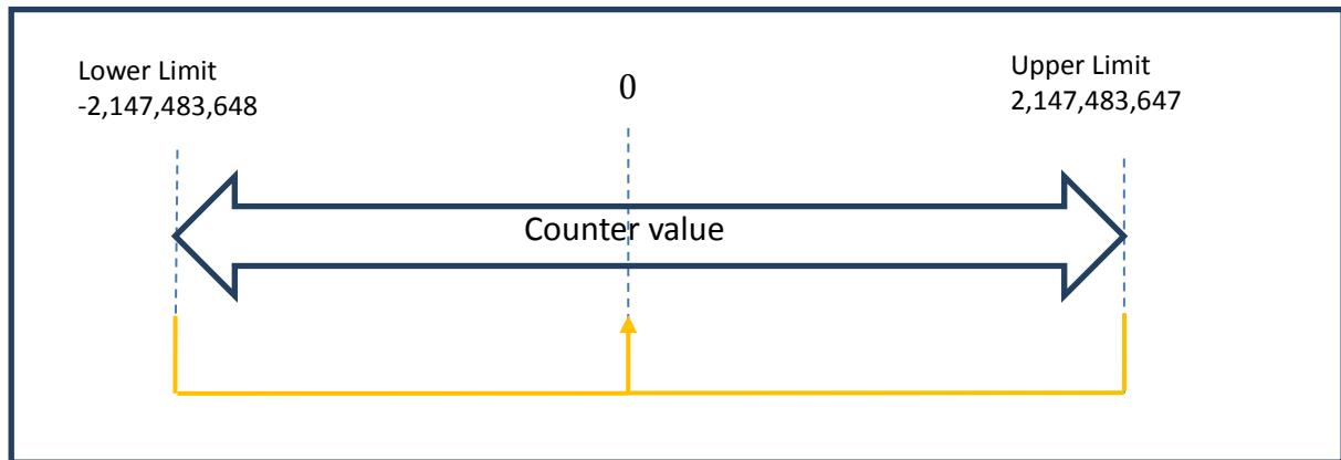
In single-pulse mode, when the upper limit is reached, the counter value will return to 0 (ring counter).
