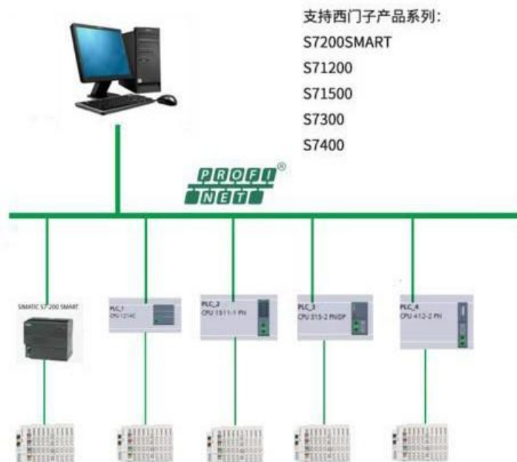
Figure 3.1 GCAN-IO-8300 Profinet bus coupler connected with Profinet controller
