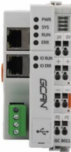
Figure 2.4 GCAN-IO-8100 module wiring terminal block
