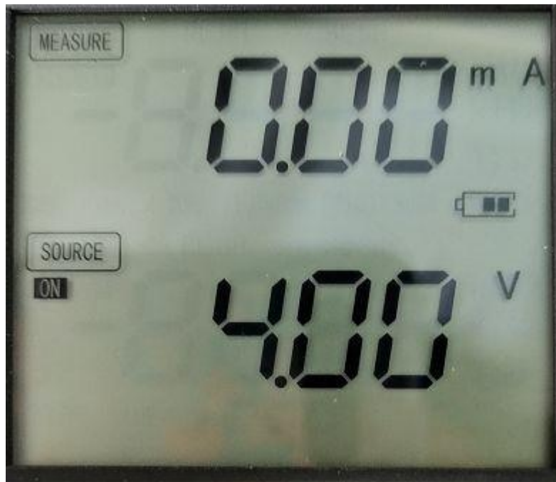
Figure 2.16 Current signal generator output voltage
